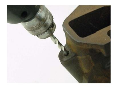
Step #4 Remove the choke stove heat element. Using the  $\frac{1}{4}$ " drift punch, Insert the punch into the previously drilled- out  $\frac{1}{4}$ " hole and press down, driving the old heat element out through the bottom fitting opening.
