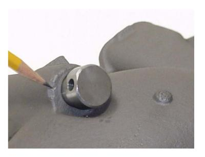
Before completing the fitting installation, make a final check to ensure the hole is lined up with the mark and the fitting is straight.
