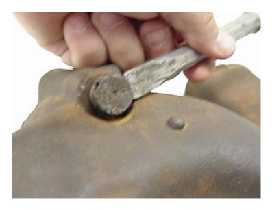
Repeat alternating back and forth until the fitting starts to move out of the manifold. Continue until the fitting is out of the manifold.
