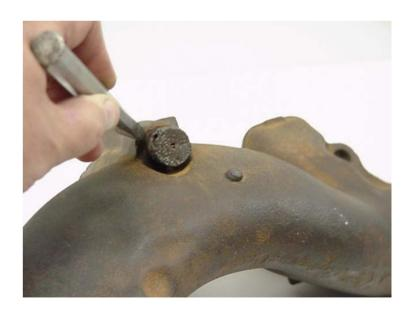
The lower fitting is held into the manifold via a pressed fit.
