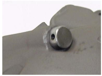
Before installing the manifolds on the engine, now is the best time to eliminate another possible problem area. I like to remove all four studs, run a tap down through the threads, and replace with new correct length & course threaded studs and four correct washer head nuts. Finally, install a set of the unique dual sized exhaust pipe donuts. on these 428 Cobra Jet manifolds.
