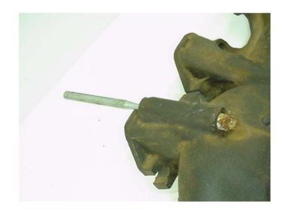
This picture clearly shows the amount of rust, scale and corrosion that came out of the choke stove chamber
