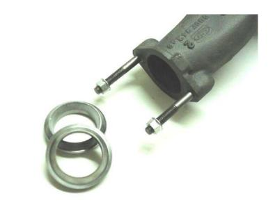
After the exhaust manifolds have been installed on the engine you can now install the plumbing. I like to use a kit as shown that includes all of the attaching hardware, woven fiberglass insulator, s-clip and pre bent hot and cold lines, made out of original equipment material.
